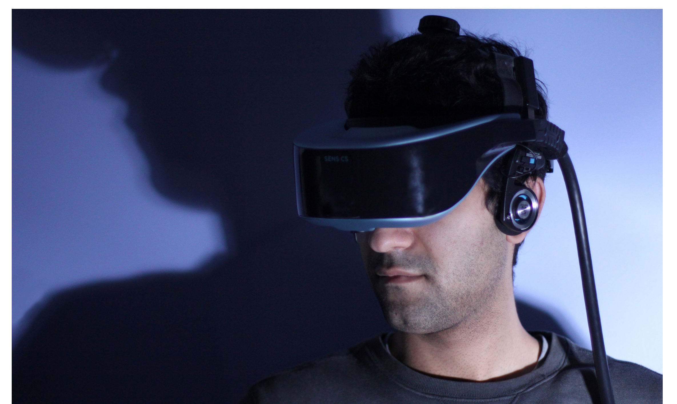
A head-mounted display from Sensics enhances a sense of immersion for the player.
